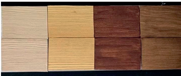
Figure 8 - Wood samples coated with NPs formulation. ISOMAT.
